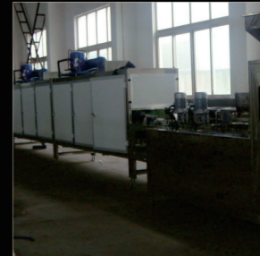
冷柜 Cooling tunnel
