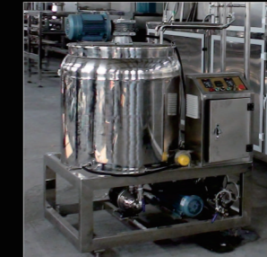
巧克力储存桶 Chocolate storage tank
